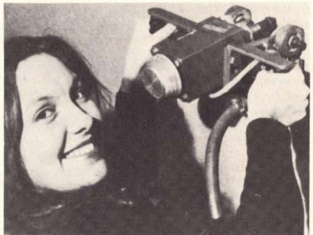
Guided along a chalk line, this new power chaser cuts grooves in wall or floor surfaces to controlled depths.
